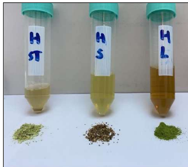
Fig. 3: Image of the powdered forms of Citrullus colocynthis plant parts (leaves, stems and seeds) placed in separate containers (lower row), along with their corresponding aqueous extracts after filtration (upper row), prepared for the green synthesis of AgNPs.
