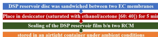
Fig. 3: Steps involved in sealing of ocuserts
