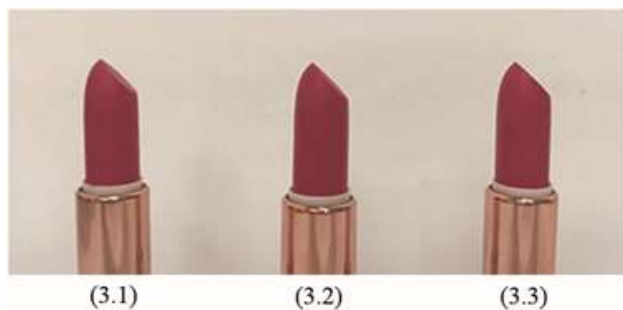
Fig. 5: Physical appearances of the obtained color lipsticks with a variation of texture enhancers (3.1) without texture enhancers, (3.2) with PMMA 4% w/w, and (3.3) with PMMA 4% w/w plus stearyl dimethicone 3% w/w
