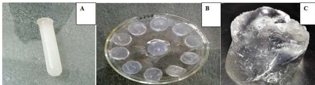
Fig. 2: Un-cut and unwashed base hydrogel (A), Hydrogel disk (B), Swell hydrogel (C)
